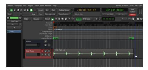
Zoom into a single impulse (Ctrl+Scroll-wheel). You will see that the impulse starts later than the gridline, which is where the red play-head is in the image below. The metronome is sounded at each quarter note on the grid, but doesn't get recorded until later, due to hardware latency. For reference the image below was taken on a system running at a buffer size of 64, and 3 periods, and shows an offset of 511 samples.
