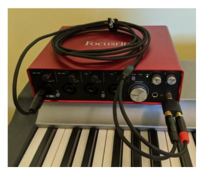
After all connections are made, jack\_iodelay will report the full loop latency, in milliseconds, frames (samples), how much of the latency is due to hardware (it does this by subtracting the known latency from the total measured), and also recommends values to set for input and output ports.
