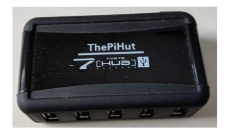
Whatever you get, Make sure it has a beefy power supply, e.g. 2A. USB WiFi dongles, particularly the ones with external antennas can be thirsty and a 2A power adapter is unlikely to cost much more than a 1A one.
